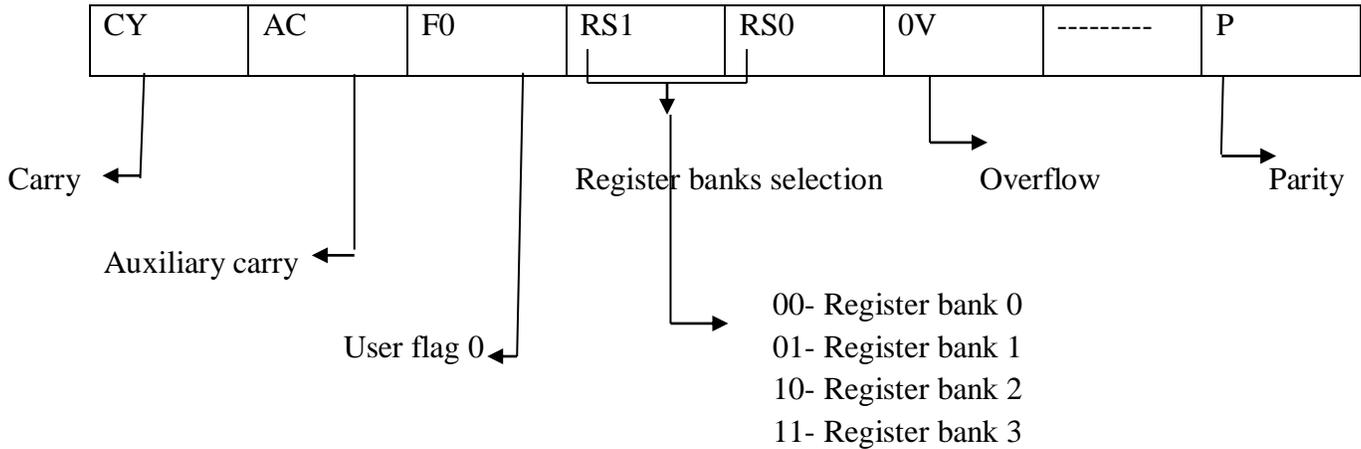
**9. State the function of RS1 and RS0 bits in the flag register of Intel 8051 microcontroller.[NOV2011]**
